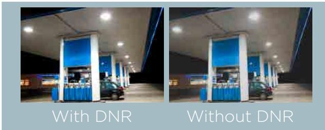
**3D Digital Noise Reduction (3D-DNR)** - Get exceptional video image quality with less noise. 3D-DNR incorporates frame-to-frame noise reduction with spatial noise reduction to produce clear video images with less noise, in low light conditions. Noise reduction is critical for video because noise affects image quality. Cameras with 3D-DNR produce sharper, more accurate video images.
