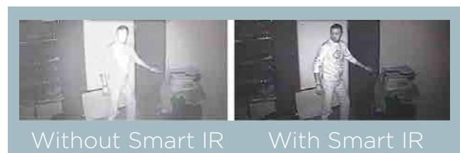
**Smart IR** – Captures clear, sharp images in low light. Smart IR (smart infrared) automatically adjusts the amount of infrared light used to illuminate a scene as the subject moves closer to or further away from the camera, resulting in optimal exposure and a sharp, clear image that is neither washed out or too dark.
